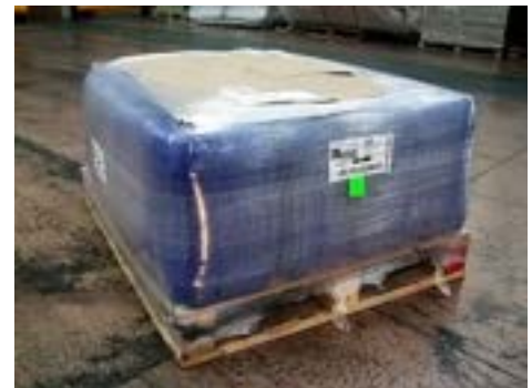
Drums, tied down and properly wrapped
