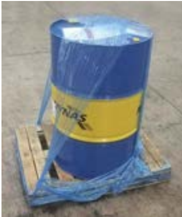
This drum is barely secured.
