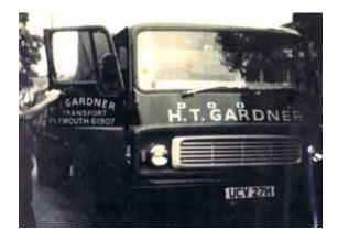
with the pride from Harold (never dad) and swelled chest and beaming smile of the driver Roger Pine. In those days the cab had to be lifted to check oil and water levels. This achieved by unscrewing two locks at the back of the cab and literally pushing the cab up and over to gain access.
